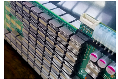
Example of today's densely packed ASIC miner boards. Each processor would need a water inlet and outlet.
